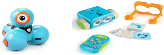
Fig. 1. The Dash robot by Wonder Workshop (left) includes sensor-based recognition and play affordances related to lights, sound, and movement. The Botley toy robot (right) operates with remote control and other accessories.
