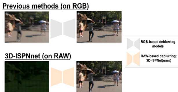
FIGURE 1. To tackle blur effect phenomenon, conventional approaches mainly rely on recursive strategies and operate in the RGB domain, whereas in this study, we promote a novel blur preventive strategy by training on sensor raw data.
