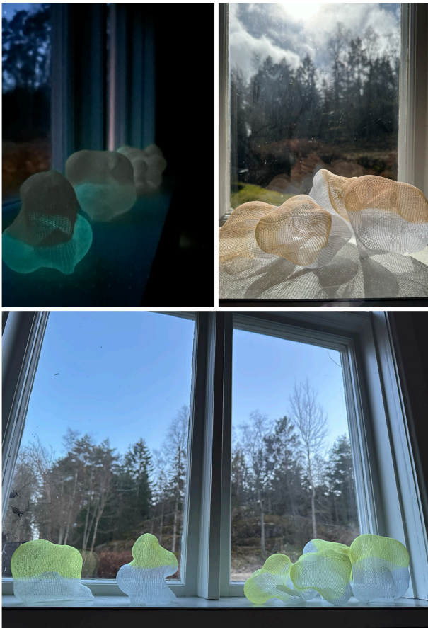
Fig. 12-14: Tubular knitted textiles demonstrating different effects of UV responsive and illuminating yarns.
