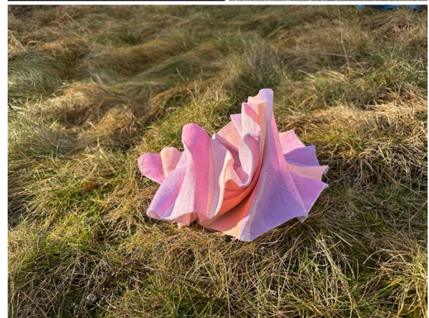
Fig. 9-11: Knitted origami textile (rosette shape) with UV-responsive and illuminating yarns viewed in darkness (9) and in daylight (10-11). Fig. 10 The folds of the origami structure have a blocking effect which causes areas of the textile to remain in its original white state.
