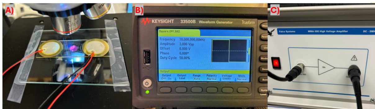
Figure 12. A) Set up for the microscope analysis. B) Waveform generator used in experiments. C) High voltage amplifier used in experiments.
