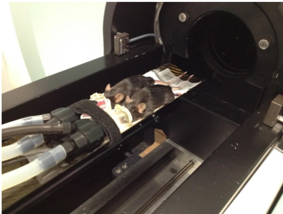
Figure 6 In animal studies (Studies I and II), imaging by PET/CT (Siemens Medical Solutions USA, Knoxville, Tenn., USA) was performed under isoflurane gas anesthesia, animals were placed in pairs in the prone position, and the ^{18}\text{F} -FDG tracer was injected into the tail vein. The author's own photograph, originally taken by Pauliina Hartiala
