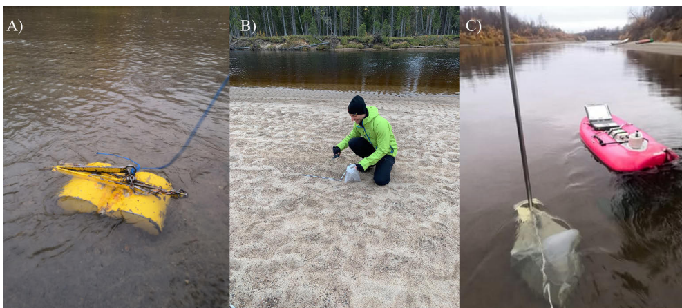
Figure 9. Collecting sediment and bedload samples. A) Van Veen grab sampler in the bottom of the river. B) Sampling point bar surface with a small spade. C) Taking bedload transport sample with a Helley-Smith sampler (left) simultaneously with stationary ADCP measurements (right).
