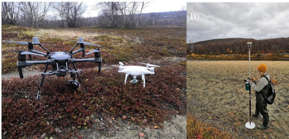
Figure 7. Collecting aerial images for the orthomosaic and mapping of bathymetry/topography with A) DJI Matrice 210 V2 RTK and DJI Phantom 4. B) Measuring GCP points with VRS-GNSS.
