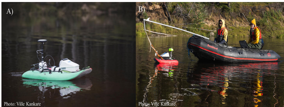
Figure 5. The ADCP attached to A) Remotely controlled platform and B) The floating platform with ADCP attached to a bow of a Zodiac.
