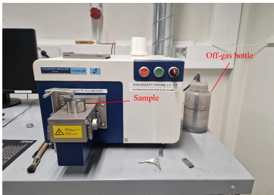
Figure 19. Measurement arrangements for OES including sample and off-gas washing bottle on the right side. The sample was placed on a spark stand and the process was operated with a computer.
