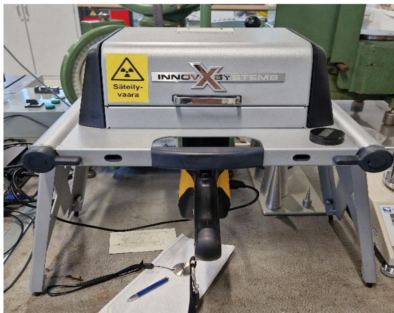
Figure 18. Measurement arrangements for XRF in desktop-mode. The 'analyzer is attached to the table stand and measurement window is pointing upwards inside the box.
