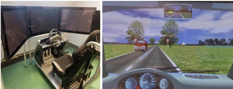
Figure 12. Driving simulator set-up. The left image shows the driving simulator used, with three of the five screens visible. On the screens, a scene was shown of which the image on the right is a screenshot during the Intersections ride of the primary screen. The primary screen is the middle screen right in front of the participant and shows what you would see through the windscreen of a normal car.
